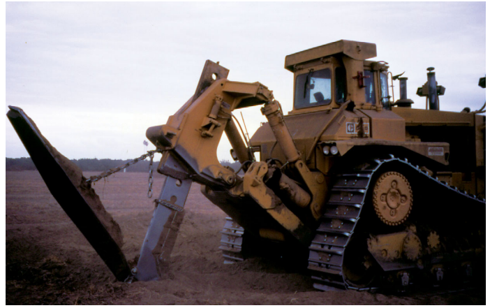
Fig. 8 Tractor with slip plow used to fracture, disrupt and modify horizons such as claypans and duripans. Credit: Kerry Arroues.
