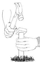
2. Move the pipe gently in a circular motion to loosen it. If the pipe is stuck, use gentle side taps with the hammer to free it. Carefully pull the pipe out of the ground, making sure the soil remains inside the pipe.
